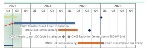
High level program of works below for EA3 converter station:
